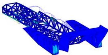
Quicksilver WSR is a world water speed craft that is currently in construction, and we have conducted the stress analysis of the frame for integrity against operating loads.
