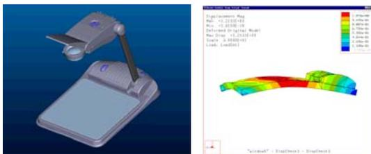
Company X had redesigned an OHP to be made from ABS instead of aluminium, only to find that it suffered from thermal distortion. They had tried some 'fixes', but none worked, so we were called in to see if we could find a solution. We analysed the model in Pro/MECHANICA Thermal and Structure, obtained correlation and then optimised the design to obtain two possible solutions; a long term one that would require a tooling change, and a short term one that didn't.
