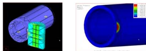
Optimisation of methodology for contact analysis of a roller on a tube.
