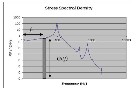
Analysis of valve mounting subject to random vibration. Then post processing of results to determine fatigue life.
